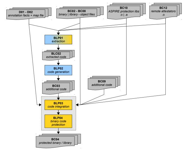
Figure 5 - Four steps of the binary part of the ACTC.
