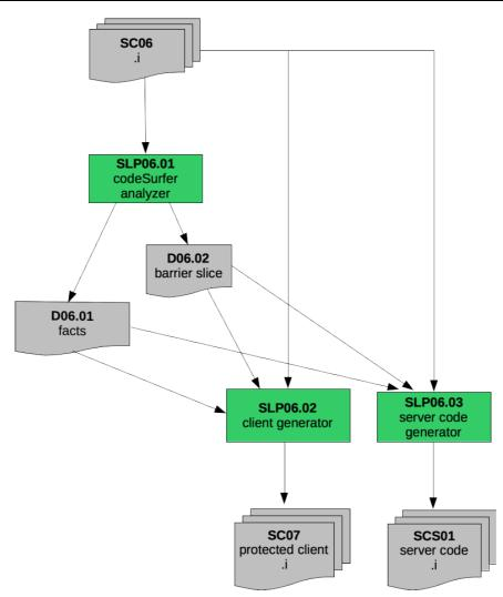
Figure 1 - Client/server code splitting tool (overview)
